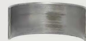
**ROD BEARINGS:** Engine bearings on an oil with low film strength and thinner viscosity can lead to premature wear or even engine failure.
