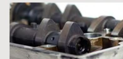
**CAMSHAFT:** Direct acting overhead camshafts are used on many Polaris engines. In this application the camshaft pushes directly on the valve, creating very high contact pressures compared to other camshaft configurations. These forces are so great that inferior oil can break down leading to increased wear and potential engine damage.
