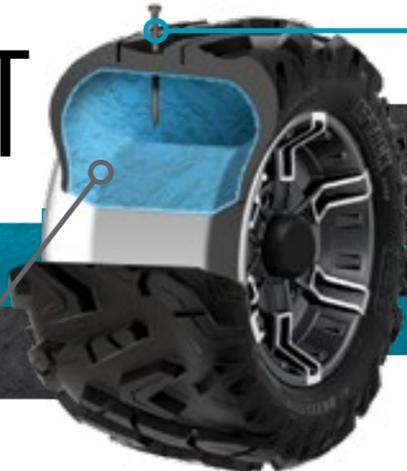
Once a leak occurs, the tire sealant rushes out of the tire and quickly creates a permanent solid plug.
