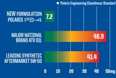
ASTM D6335. In 3rd party against 9 competitive products Polaris PS-4 had less than half the deposits compared to the next closest product. No other tested products met Polaris Engineering standards for deposit cleanliness.
