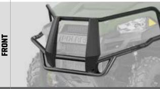
**1 ¼" DIAMETER** STEEL TUBE CONSTRUCTION
