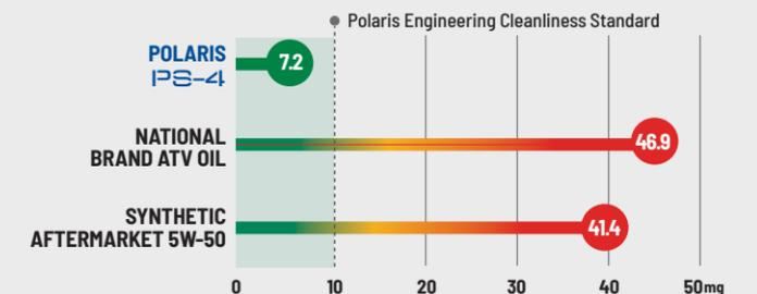
ASTM D6335. In 3rd party testing against 9 competitive products Polaris PS-4 had less than half the deposits compared to the next closest product. No other tested products met Polaris Engineering standards for deposit cleanliness. Test measures mass of deposits in mg in high temp, high stress test cycles. Higher deposits will impact engine power and performance.
