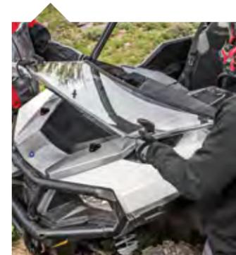
Offers fully-sealed or flipped-down venting options. Upper half detaches, leaving lower half for protection with maximum ventilation.
