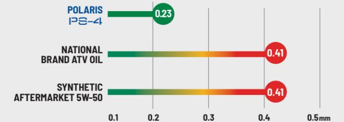
ASTM D4172. In 3rd party testing against 9 competitive products Polaris had 40% or better wear protection compared to all of the tested products. Numbers represent mm of wear scarring measured. Test measures wear at contact points, wear scar is measured for its length and width (in units of mm). Lower wear numbers mean better wear protection and friction reduction.
