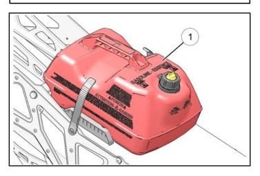
7. Place fuel can cover over installed fuel can ensuring cover mates with the contour of the fuel can properly.
