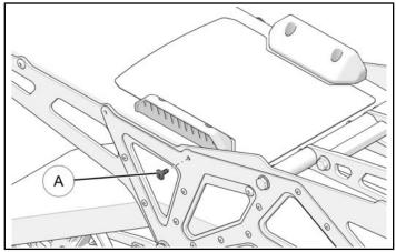
5. Using provided screw ⑦ and locking nut ⑧, install ratchet ladder straps ④ to the outside of the left and right side panel. Torque to specification.
