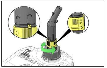
4. The spout has two molded hook features seen below that allow the fuel spout to be pushed down against the receiving container to compress the spring mechanism of the spout and allow the fuel to flow through the spout.
