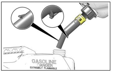
Place end of spout into receiving container with one of the hooks firmly against the lip of the receiving container push down on the fuel can to compress the spring mechanism and allow the fuel to flow.
