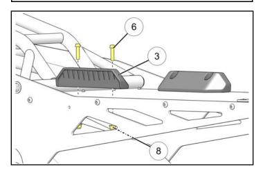
6. Install gas mat with larger area of mat towards the rear of the vehicle.
