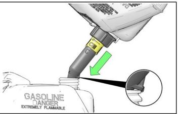
5. When receiving container is near full, slowly pull back the fuel can while keeping the end of the spout in the receiving container to avoid spilling gas. This will allow the spring loaded mechanism of the spout to extend back to the original position and stop the flow of fuel.
