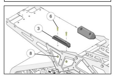
3. Ensure top of tunnel is clean and free of debris. Remove protective paper to reveal the adhesive backing on the gas mat and install gas mat with larger area of mat towards the rear of the vehicle as shown.
