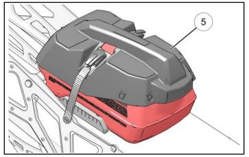
Insert left and right side ladder straps ④ into the ratcheting buckles ⑧ on the fuel can cover ⑤. Ratchet both buckles equally on both sides until fuel can is tightly captured and secured with no movement of the fuel can.
