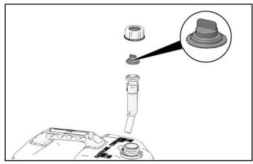
2. Reverse direction of spout, place spout back onto fuel container, install the cap over the top of spout and screw cap back onto threaded portion of container making sure the spout is firmly seated onto the container and the cap is tight.
