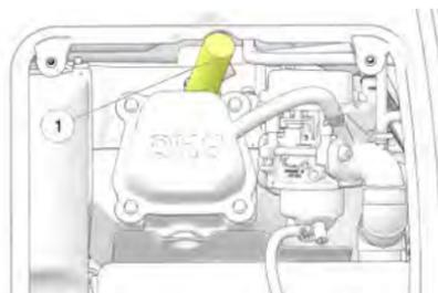
8. Re-install the spark plug cap ①.
