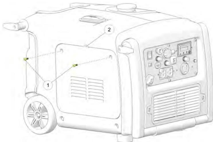
5. Upon completion of maintenance, replace cover by inserting the bottom edge into the grooves and replacing the two screws.
