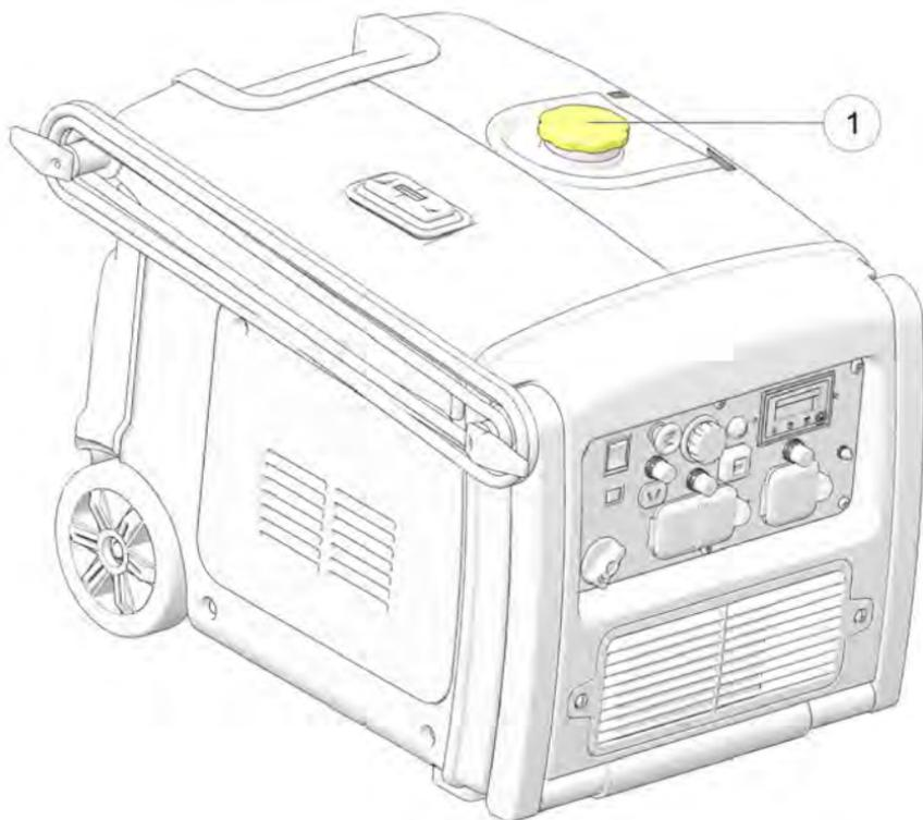
5. Position fuel switch to OFF for storage or ON to operate the generator.
