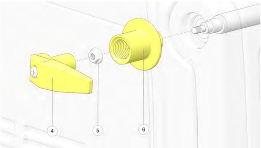
4. Secure base with hex nut ⑤ using a socket wrench.
