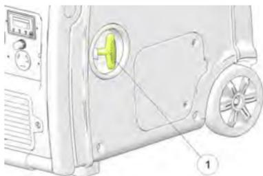
2. For a cold engine start, pull out the choke lever (if equipped) to CLOSED position.
