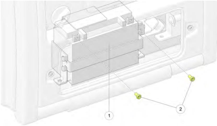
5. Disconnect the black (negative) battery cable first by removing the M5 screw ②.
