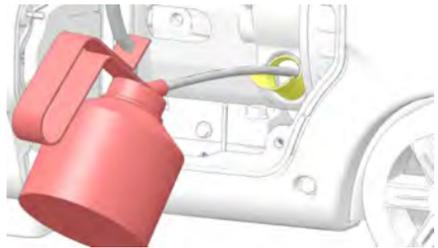
4. Insert the dipstick into the filler neck, without screwing it in.
