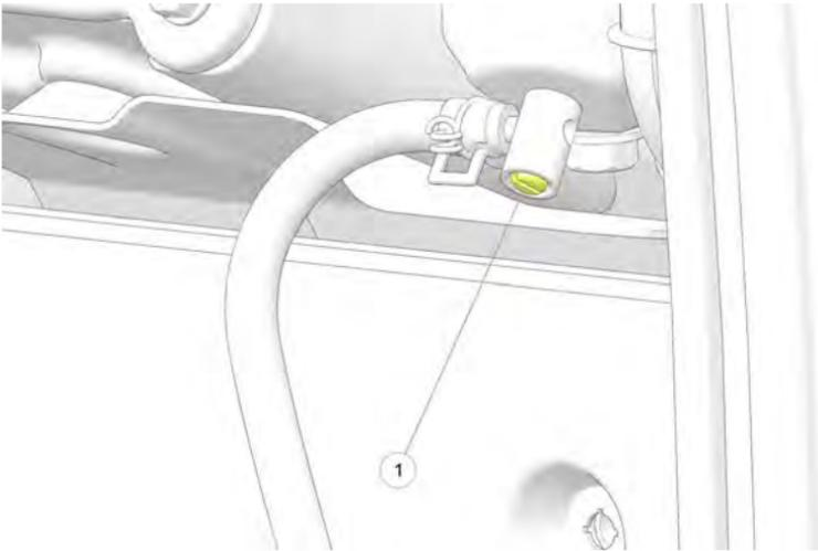
8. Turn fuel valve switch to ON and drain gasoline into pan.
