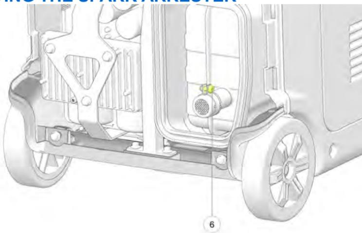
1. Remove screw ⑥ holding the spark arrester to the muffler.
