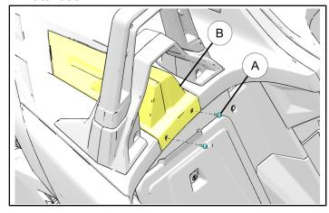
3. Carefully pull the RH panel (B) up, starting from the front and working back until the entire panel is removed.
