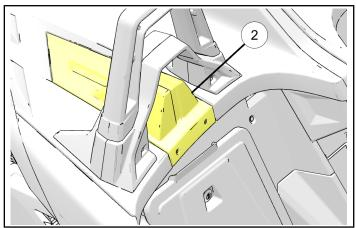
2. Use an M4 Allen Wrench to re-install the bolts (A) at the front of the panel ②. Removed in Step 2 (Section - Removal of Rear Deck Hump Panel).
