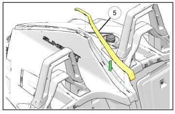
2. Work from the back towards the front of the vehicle, firmly press on the trim ⑤. Ensure the tabs engage.
