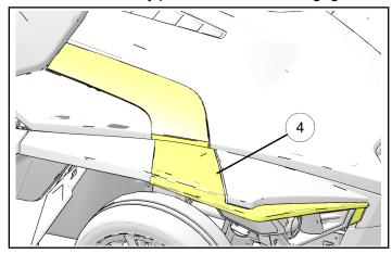
Using a T25 Torx® wrench install the screw (F) located in the front tip of the panel adjacent to the light.
