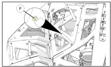
3. Remove one screw (F) from the front tip of the panel (G) by using a T25 Torx® wrench. Retain the screw for later use.
