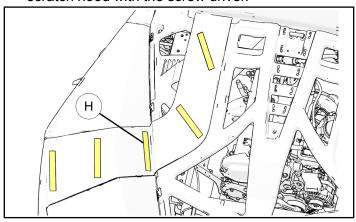
6. Finish removing the panel (G) by carefully pulling the component from its front tip working backward towards the rear. There are three molded tabs (J) that must be dis-engaged above the front light.
