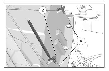
4. Drill hole through topside of each upper dash tab.
