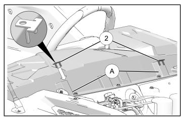
2. Use mount (2) as a template to mark holes on each upper dash tab (A).
