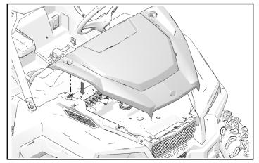
2. Rotate latches 90° to lock hood into place.
