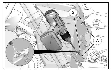
5. Install two windshield support mounts 2 to upper dash tabs A using two push pin rivets 3.
