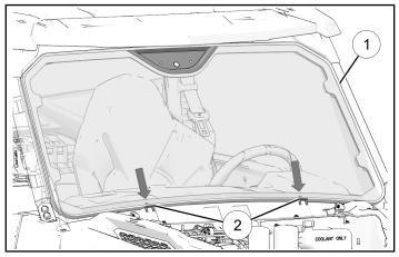
3. Push four windshield clamps to locked position on ROPS.
