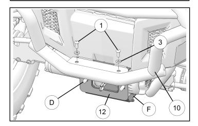
6. Run winch cable through the fairlead (E) and install fairlead onto screws (D) at the front sandwiching winch adapter bracket ② as shown. Install washers ③ and nuts ⑤ to secure fairlead in place. Don't tighten fasteners at this time.
