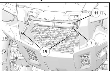
4. Align and install upper part of the bumper weldment <sup>®</sup> onto mounting bracket <sup>®</sup> using two socket head cap screws <sup>®</sup> and two lock washers <sup>®</sup>. Don't tighten fasteners at this time.
