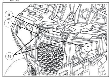
7. Align and install upper part of the bumper onto mounting bracket ① using two socket head cap screws ③ and two lock washers ①. Align and install lower part of the bumper onto bumper bracket ④ using two button head socket cap screws ① and two flat washers ③. Don't tighten fasteners at this time.
