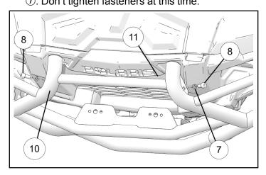
Align mounting holes on lower part of bumper weldment (1) with top holes on winch adapter bracket (1) and install two screws (1) and washers
