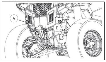
5. Install bumper bracket (4) onto frame bracket (3) using four button head socket cap screws (1) and four flat washers (3). Don't tighten fasteners at this time.
