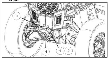
6. Install mounting bracket ① to vehicle using two self-tapping bolts ⑤ and two lock washers ② provided in the kit. Don't tighten fasteners at this time.
