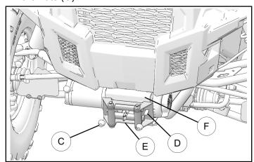
3. Install mounting bracket ① onto vehicle using two self-tapping bolts ⑤ and lock washers ⑦ provided in the kit. Don't tighten fasteners at this time.
