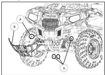
3. Install frame bracket ③ onto chassis bracket by aligning holes and fasten using four hex bolts ⑥, flat washers ④, and lock washers ⑨ as shown. Don't tighten fasteners at this time.
