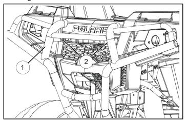
Align brushguard lower mounting bracket holes with holes on welded hitch assembly and install four screws (4) and nuts (5). Tighten screws to specifications.
