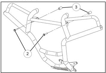
Align and install upper portion of rear brushguard assembly 1 to the vehicle by installing screws 2 as shown. Install screws well enough to hold the brushguard in place. Tighten the screws until snug.
