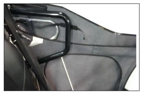
17. Tightly close the RHS door and adjust Insert the ½" webbing strap (20) with the red webbing handle through the channel on the doors from front to back. Screw the ½" webbing strap to the latch using the supplied screw, threading it into the supplied knob (18).
