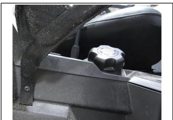
5. Unbuckle and remove net from rear ROPS tube on both sides of vehicle.
