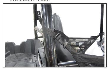
6. Remove existing side bolster bars from vehicle by removing two bolts on each bolster bar. Retain hardware for later use.
