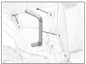
4. Install the bolster bar bracket (2) on bolster bar (E) using screw (2) and hexagonal flange nut (6). Do not tighten at this time.
