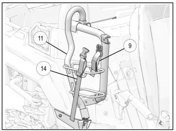
9. Adjust webbing to hold gun boot securely in place.
