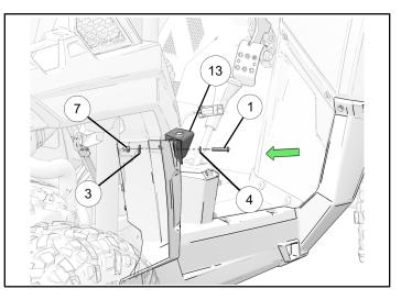
6. Install gun scabbard mount (1) onto fender bracket (3) by inserting pin (6) through rubber grommet (8).
