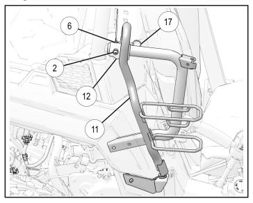
8. Install female webbing assembly (a) and male webbing assembly (a) on the gun scabbard mount (1). Insert gun boot and secure with webbing and buckles.
