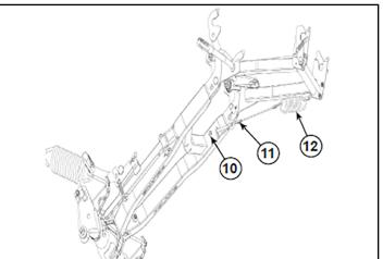
3. Refer to the Plow Frame (2879630) installation guide for the proper height adjustment procedure.
