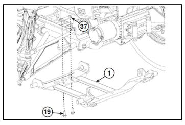
5. Fasten the front lower area of mount plate to the machine using two M10-1.25 X 35 mm hex bolts (6), two lock washers (2), two flat washers (3) and two front tightening plates (3). Assemble the mount plate to the square tube assembly that was installed in Step 2 with two M8-1.25 X 25 mm carriage bolts and two nylon flange nuts (0). All hardware should be hand tight at this time.
