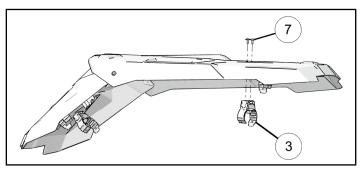
b. For cab frame extension models, drill two holes on rear roof and install clamps ③ by inserting screws ⑦. Do not tighten at this time. Refer kit drawing on first page for hole locations. Install two plastic darts ⑥ in the molded holes to seal them.
