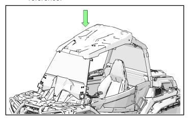
b. For cab frame extension models: Put pressure directly over clamps as shown. See direction arrow for reference.
