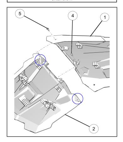
b. For cab frame extension models, align front holes (as shown) on rear roof ② with front roof holes and install screws ④ and Tuflock® rivets ⑤.
