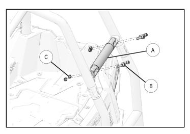
Install spare rear tire weld mount ① in location where center link tube was removed using screws (B) and nuts (C). Ensure that center tire support tube faces out away from vehicle (toward the rear). Torque fasteners to below specifications.
