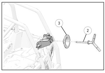
4. Check spare tire weld mount at every stop or every 50 miles to ensure tire handle assembly is still secure. Check tightness of all fasteners on cab frame extension and tire weld mount before and after each ride.
