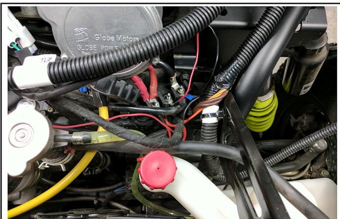
3. Secure all remaining wires to the to the vehicle at this time using supplied cable ties.
