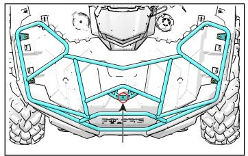
5. After drilling new mounting hole, open front storage box cover to gain access to the underside. Use provided screw (2) and nut (3) to secure center rack mount into position.
