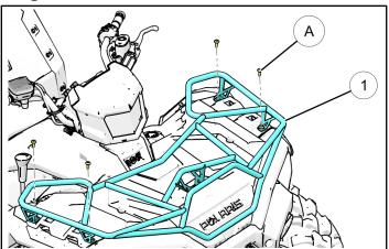
4. Once you have secured the rack you will need to use a drill and 1/4" drill bit to make a new hole for fastening the center support of the rack to the front storage box cover in the location indicated below.
