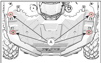
3. Place rack on front storage box cover, align mounting holes and fasten using existing screws (A)
