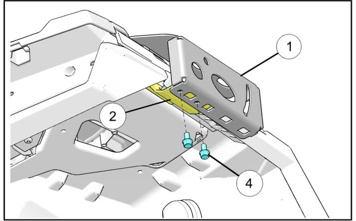
5. Insert previously installed screws (A) through lower gun mount bracket holes and install retained nuts (B). Tighten screws (A) and ④ to below specification.
