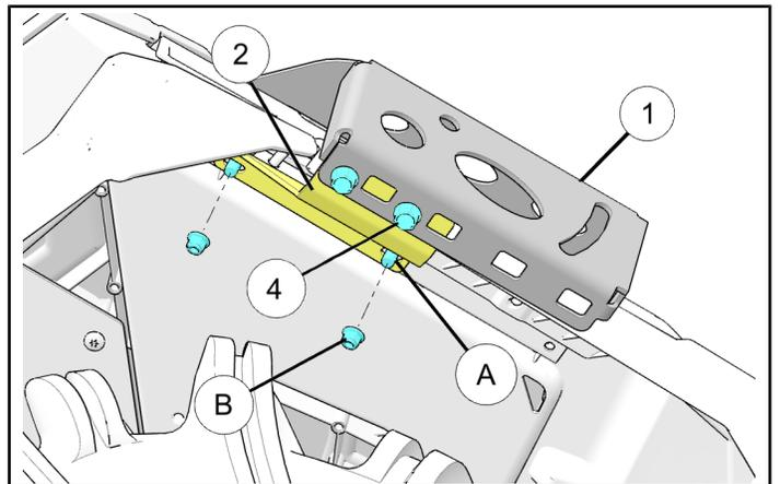
6. Install quick latch bracket ③ onto upper gun mount bracket ① using two screws ⑤. Install nut ⑥ on the front screw as shown. Torque screws ⑤ to below specification.
