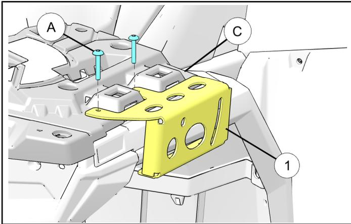
4. Install lower gun mount bracket ② onto the upper gun mount bracket ① by aligning holes and installing two screws ④ as shown. Do not tighten hardware at this time.
