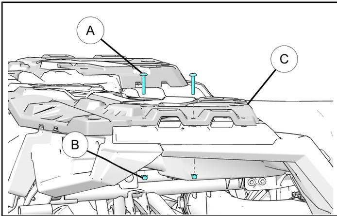
3. Loosely install upper gun mount bracket ① to the rear rack (C) using retained screws (A) as shown. Do not install nuts (B) at this time.
