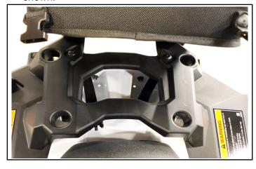
2. Route the attachment straps under the rear rack support tube to the front of the rack as shown.
