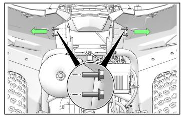
3. Torque all four mounting screws to specification.
