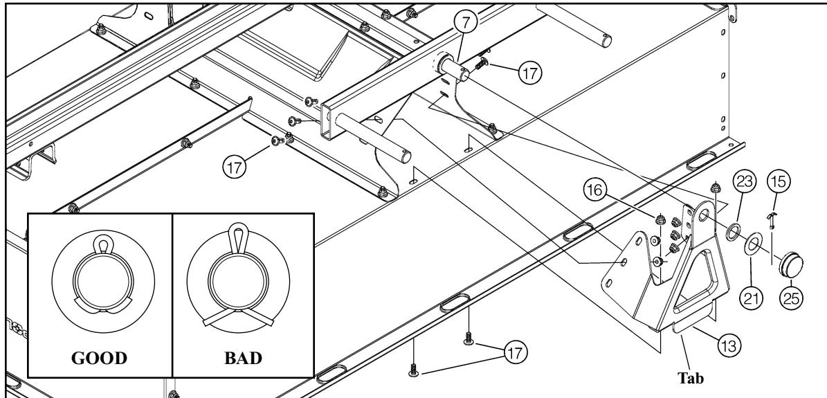
6. Insert the 46mm X 26mm X 1.5mm shim (#21), the sleeve (#22), the wheel (#14), the 35mm X 26mm X 3mm shim (#23), and the 46mm X 26mm X 1.5mm shim (#21) on each axle of the swingarm (#8). Insert the 4.5mm cotter pin (#15) at the end of the main axle (#8) (make sure that the cotter pin does not exceed the diameter of the shim (#21) once folded in place) and install the plastic cap (#25) on each axle of the swingarm (#8). Verify that the tire pressure is correct.
