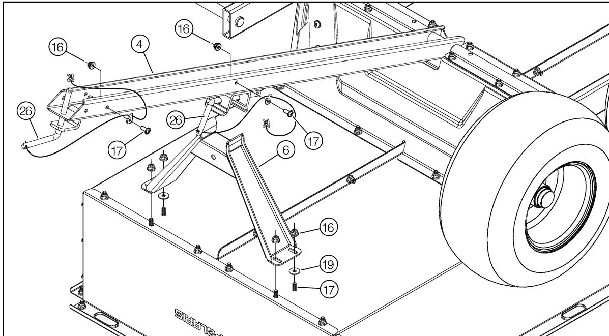
8. Position and fasten the rear right (#10) and left reinforcements (#11) onto the box (used the pivot holes of the rear panel as reference) using (12) M8-1.25 X 20mm Allen socket machine screws (#17) and (12) M8-1.25 nylock flange nuts (#16) (do not tighten at this time).
