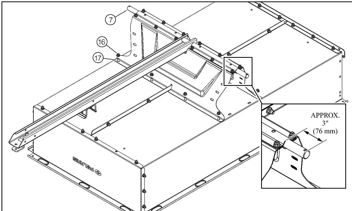
4. Apply some grease on the main axle (#7). Slide the 45mm X 26mm X 1.5mm shim (#21) and the swingarm assembly (#8) on the main axle (#7). **Note :** It is suggested to re-grease occasionally.
