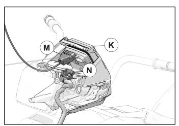
15. Route the GPS receiver harness (1) properly and connect to the vehicle diagnostic and main harness as shown in figure.
