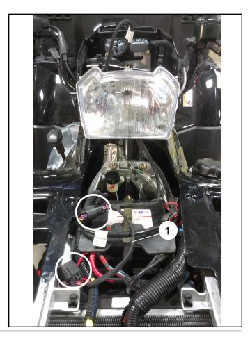
16. Route the USB harness (P) properly and tie with handlebar as shown in figure.
