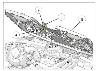
4. Place front rack onto its original position and lock the lock and ride anchor.
