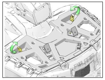
5. Install front audio mount bar ① onto weld bracket mount by using two M8 screws ②, spacer ⑤ and nuts ③.
