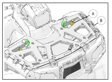
2. Line up upper brackets as shown and use the brackets as a template to mark the holes in the rack. Lift up the rack to avoid drilling into the storage compartment underneath the rack. Drill holes with an 8mm or 5/16" drill.
