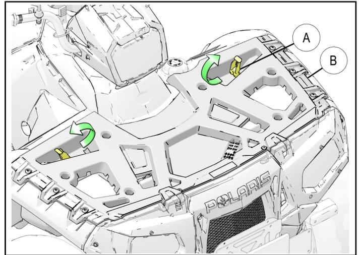
2. Line up upper brackets as shown and use the brackets as a template to mark the holes in the rack. Lift up the rack to avoid drilling into the storage compartment underneath the rack. Drill holes with an 8mm or 5/16" drill.
