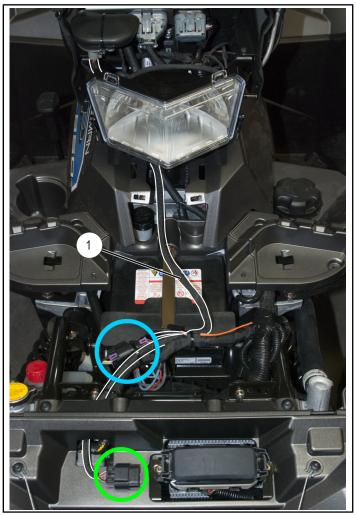
15. Route USB harness ⑥ and attach it to handlebar using Panduit strap as shown.
