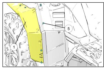
8. Align rear LH fender flare ② with vehicle body panel (H) as shown. Using existing holes on fender flare as templates, mark three holes on body panel in the locations as shown.
