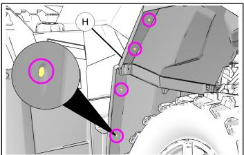
5. Align front LH fender flare ① with vehicle body panel (G) as shown. Using existing holes on fender flare as templates, mark three holes on body panel in the locations as shown.
