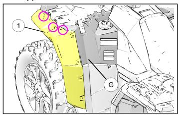
6. Drill three holes in the marked location on vehicle body panel (G) using 5/16" drill bit.
