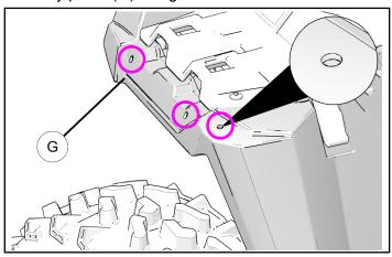
7. Align and install front LH fender flare ① on vehicle body panel using seven tuflok rivets ⑤ as shown. Repeat same on other side of vehicle.
