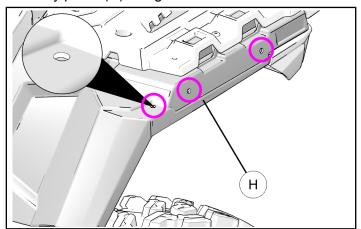
10. Align and install rear LH fender flare ② on vehicle body panel using seven tuflok rivets ⑤ as shown. Repeat same on other side of vehicle.
