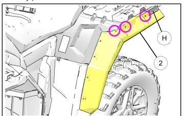
9. Drill three holes in the marked location on vehicle body panel (H) using 5/16" drill bit.
