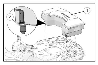
5. Once in place, secure the rear cooler into position by rotating the Lock & Ride anchor handles **2.1** down into the locked (horizontal) position as seen in the image below.
