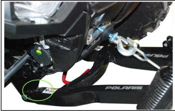
9. Pull the locking handle © UP TO LOCK the plow in place on the ATV frame.
