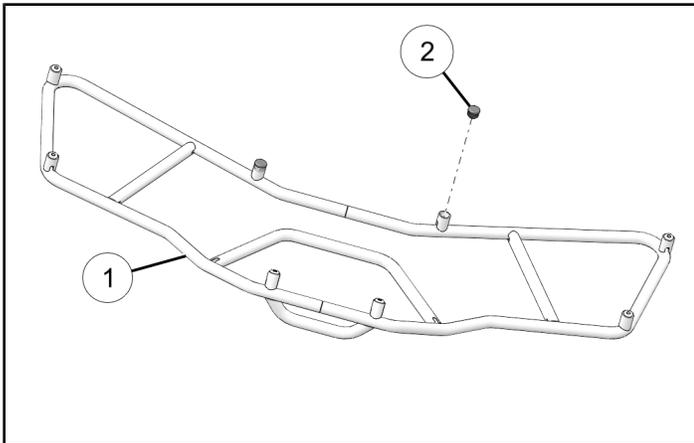
2. Open front box cover and align utility rack pins with holes in cover.
