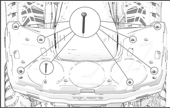
2. Align rear utility rack. Install all eight screws and nuts.
