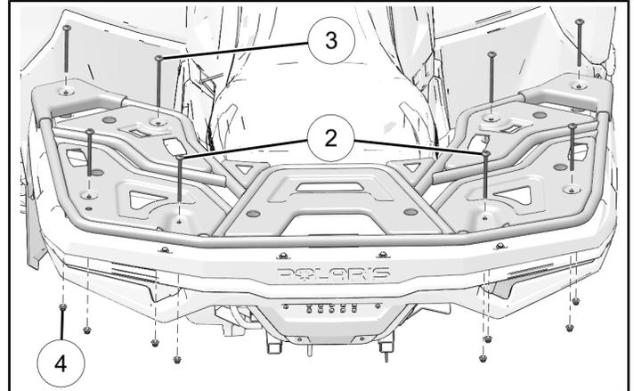
3. Counter-hold nuts and torque all screws to specification.
