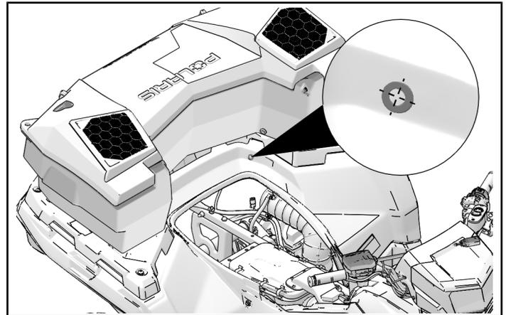
3. Insert wire harness connector through hole and install grommet 1.6 into hole.
