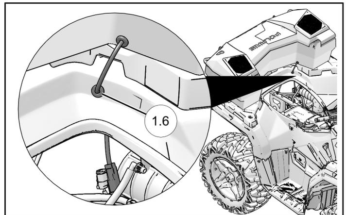
4. Connect wire harness connector from audio rear storage box to rear accessory power harness connector (sold separately).
