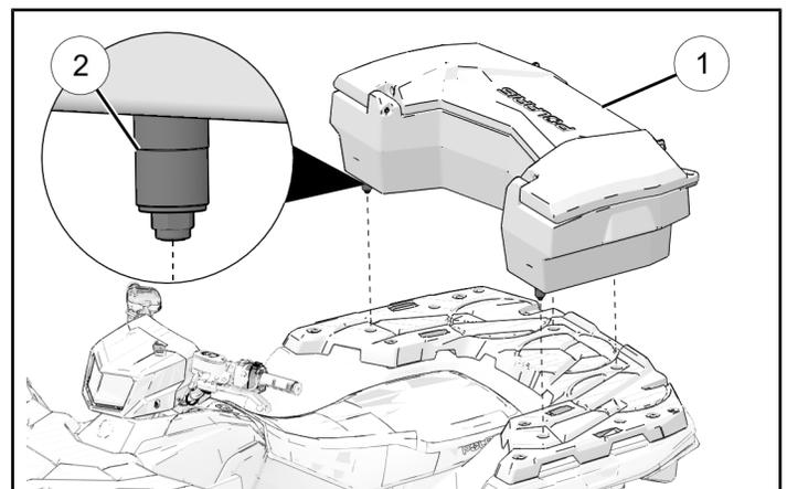
5. Attach rear storage box by rotating Lock & Ride anchor handles down into the locked (horizontal) position as shown.
