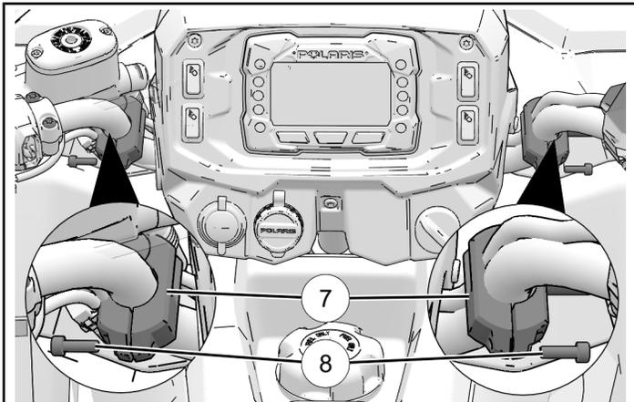
4. Install the windshield assembly onto the mounting clamps and take time to position the mounting clamps and adjust the windshield to the headlight pod. Tighten both windshield mount adjuster screws and torque the mounting arm fasteners ⑥ and mounting clamp fasteners ⑧ to specification once the windshield is in place.
