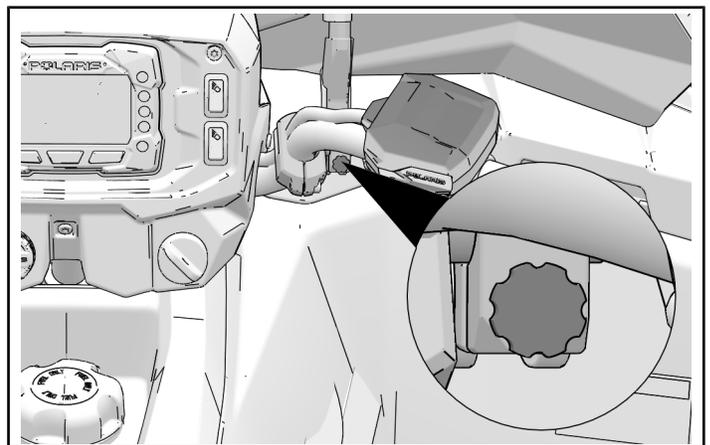
2. To optimize windshield fit, remove the mount covers and loosen fasteners on the inside of the windshield. Adjust as needed and torque fasteners to specification. Reinstall the mount covers.
