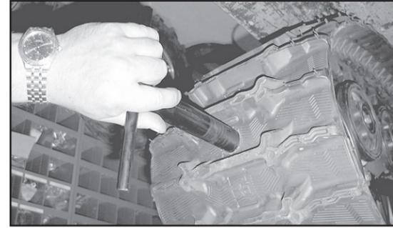
Figure 30 - Removal of the adjustment bolt
