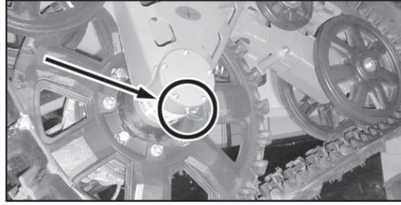
Figure 25 - Front track main axle greasing location
