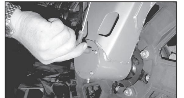
4. Remove the bearing cap using a 1/8" Allen key, taking care not to damage the cap.
