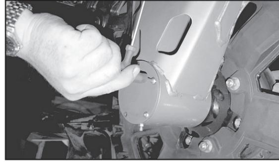
Figure 38 - Removal of the bearing cap
