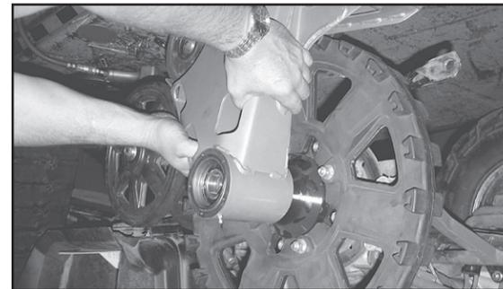
6. Pull on the frame as straight as possible to remove from the main axle.
