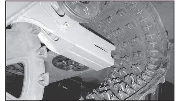
Figure 44 - Track adjuster removed
