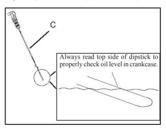
NOTE: A rising oil level between checks in cool weather driving can indicate contaminants such as gas or moisture collecting in the crankcase. If the oil level is over the full mark, change the oil immediately.
