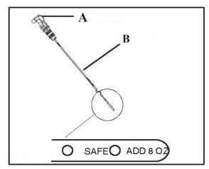
5. Reinstall dipstick and push it into place. Do not lock the dipstick.
