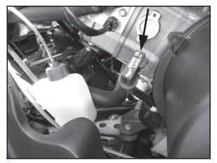
4. Unlock the lever lock (A). Remove dipstick (B) and wipe dry with a clean cloth.
