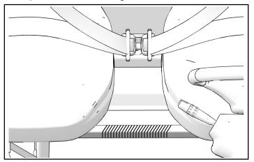
3. Join two Velcro pads ② together, remove backing from one side and place in the following locations after wiping the locations with rubbing alcohol to assure a clean surface.
