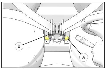
2. Clean front seat base rail area (shown with hatch lines) thoroughly with soap and warm water and wipe down with rubbing alcohol.
