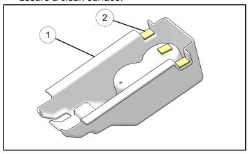
4. Remove backing from other side and place between seats being careful that the center section of the console ① is tucked under the seat belt buckle mounting bracket (C). Press down firmly at each of the mounting locations.
