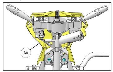
16. Remove the steering column weldment (AB) by removing four bolts to the front steel dash frame with 13mm socket and ratchet and unhook the turn stalks and ignition. The key must be in the ignition to disengage the steering lock for removing the steering column.
