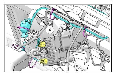
33. Route EPS battery harness as EPS battery (+ve) ® to BMC (+ve) and EPS battery (-ve) <sup>(1)</sup> to BMC V (-ve). Remove main harness +12V cable from BMC (AE) can zip tie back to main harness (this will not be connected anymore with this option).
