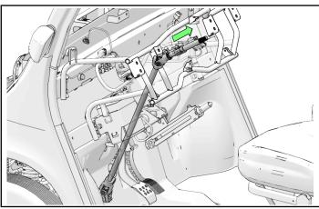
18. Install six rivnuts (4) with rivnut gun for supporting the EPS and EPS battery.
