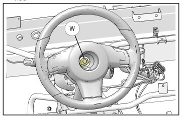
11. Remove steering wheel using a punch and hammer. Center the punch on the steering shaft and make sure the steering wheel nut (W) is still on to prevent damage to steering shaft threads. Strike the punch until you feel the steering wheel pop off of the steering shaft taper (usually this takes a large amount of force).
