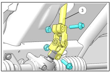
23. Install bearing and bushing on the upper steering shaft ① as shown below. Torque down the U-joint bolt ⑩ and nut ③ with 15mm socket and ratchet and 17mm wrench.
