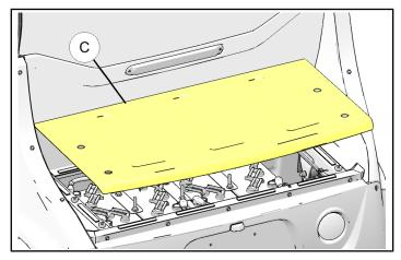
For eL XD: Remove six socket head screws
