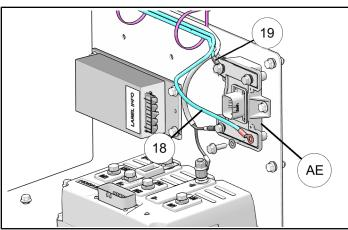
34. Disconnect the +12V battery cable from the rear battery pack and tie it off with a zip tie (this will not be connected anymore with this option). Use 1/2" socket and ratchet if removing the flooded battery pack. 13mm socket and ratchet if replacing the maintenance free pack.
