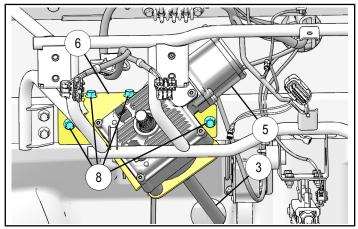
22. Tighten the lower steering shaft ③ with 15mm socket and ratchet and 17mm wrench. Start with the lowest bolt first. Once the lower joint is torqued, proceed to torque the slip joint as well.
