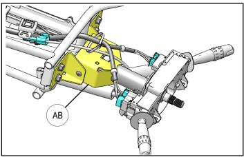
17. Remove lower steering shaft bolts with 15mm socket and ratchet and 17mm wrench and remove the fixed steering shaft (AC) by pulling it through the splash guard towards the driver's seat as shown.
