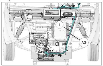
31. Plug in the EPS harness ④ to the diagnostic port in the front harness (AG) and replace the diagnostic port location with the other connector in the EPS harness.
