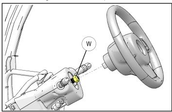
12. Remove the steering wheel nut and steering wheel and set aside. Be careful to not break the self-cancelling turn signal tab (X) on the back of the steering wheel.
