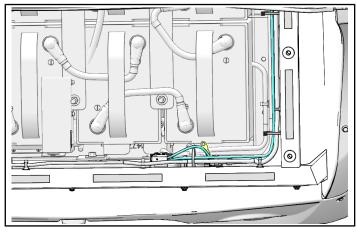
35. Install relay 16 to the fuse box as shown.
