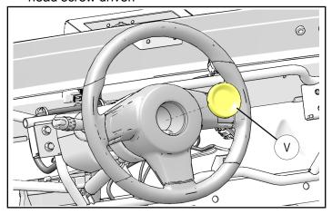
10. Loosen steering wheel nut (W) by using15/16" socket and ratchet and extension but leave 2-3 threads engaged to the steering shaft for the next step. Make sure key is out of the ignition as it will help to use the steering lock to loosen the steering nut.
