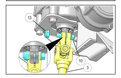
21. Install EPS ⑤ with bracket ⑥ and shaft ③ into the vehicle and tighten using four bolts ⑧. Slip the steering shaft onto the rack during install. Tighten bolts with 13mm socket and ratchet. Torque to specification.
