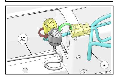
32. Plug EPS harness ④ into the EPS. Zip tie ① relay and harness.
