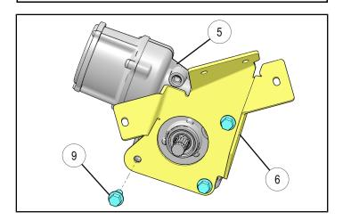
20. Install lower EPS steering shaft ③ to EPS with screw ⑩ and nut ③ outside of vehicle. Make sure to align the slit on the knuckle with the skip tooth on the steering rack. Tighten the screw and nut with 15mm socket and ratchet and 17mm wrench. Torque to specification.
