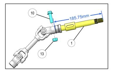
24. Install steering column weldment (AB) to steering shaft ① and install the assembly back to the steel dash frame using four bolts. and 13mm socket and ratchet. While installing slip the steering shaft onto the EPS and ensure the skip tooth is aligned with the slit on the U-joint. The U-joint slits should align when installed.
