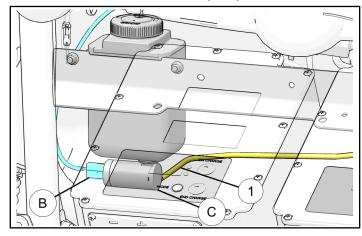
2. Install washer bottle ② to frame with screws ⑦ and nuts ⑧ using 10mm socket with ratchet and 10mm wrench. Torque nuts to specification.
