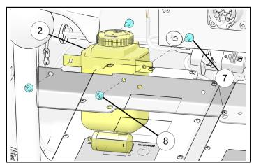
4. Route the washer hose ① through front electrical harness as shown below. Ensure there is enough hose for the wiper arm to fully function and not interfere with the with the parking brake lever.
