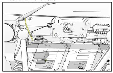
5. Install two hose clips ④ onto washer hose ① and then install the clips onto the wiper arm (D) using the flat head screw driver. Make sure the clips are on the locations shown on the spring. Improper location may cause clips to break.
