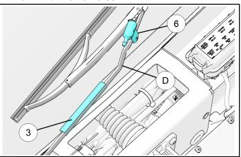
7. Finish routing washer hose ① through the hose channel ③ and attach to the nozzle ⑤/⑥. Trim excess hose length after a dry test run. Ensure no binding in the hose.
