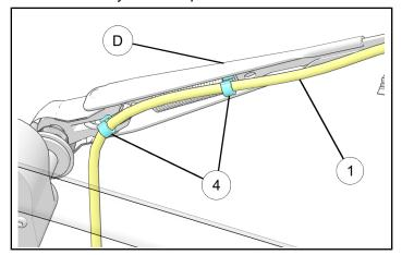
6. Install wiper hose channel ③ to wiper arm (D) and install washer nozzle ⑤/⑥ to the wiper arm using Phillips screw driver.
