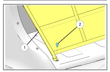
4. Install roll-in nuts ④ into OPS T-slot. Use flat head screwdriver underneath to prevent nut from sliding out and to ensure nut is centered in the T-slot. Install net using screws ③ and washers ⑤. Use T40 socket and torque wrench for tightening. Torque screws to specification.
