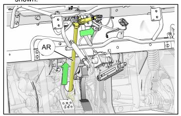
22. Remove nut (8) and bolt (11) from upper steering shaft joint. Slide upper shaft (14) from joint.
