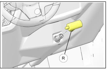
9. Remove five push-pin rivets @ from lower dash panel P.
