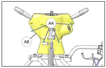
17. Remove two screws @. Remove upper steering column cover @.
