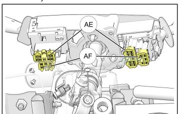
19. Install key in ignition and turn to "ON" position to disengage steering lock. Remove four bolts @. Remove the steering column weldment @from the front steel dash frame.
