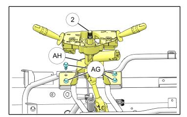
32. Loosely install bolt ① and nut ② into upper shaft joint but **DO NOT TIGHTEN**
