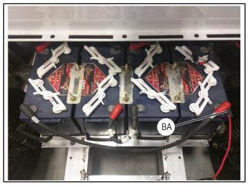
44. Route EPS battery harness (9) and (20) from EPS battery (18) to BMC .
