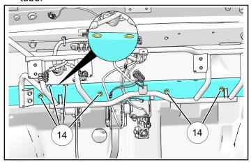
25. Outside of vehicle, install EPS mounting plate 6 to EPS ④ using three bolts ⑨. Torque to specification.
