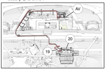
45. Remove main harness +12V cable (BB) from BMC (AV). Cable tie back to main harness (this will not be connected anymore with this option).
