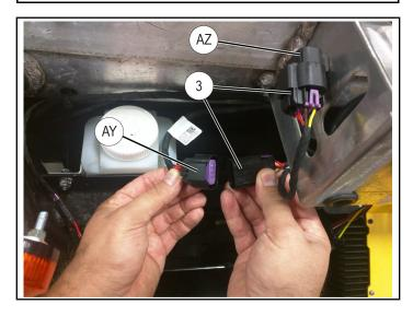
42. Plug EPS harness ③ into EPS ④. Cable tie ⑦ relay and harness.
