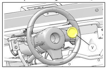
12. Loosen steering wheel nut (w) leaving 2-3 threads engaged to steering shaft for next step. Make sure key is out of ignition as it will help to use steering lock to loosen steering nut.
