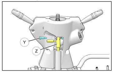
16. Remove four screws (49), lower steering column cover (48).
