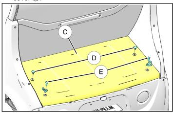
For eL XD: Remove six hex head screws (1) and three screws (1) to remove rear battery access cover (1).
