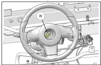
13. Center punch on steering shaft and make sure steering wheel nut (w) is still on to prevent damage to steering shaft threads. Strike punch until you feel steering wheel pop off of steering shaft taper (usually this takes a large amount of force).
