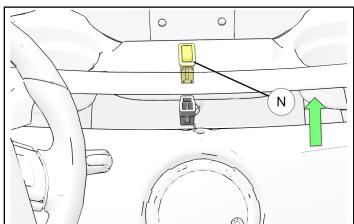
7. Remove screw from parking brake handle ®.
