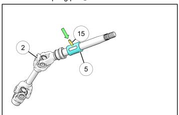
31. Install steering column shaft ② into steering column weldment � and install assembly back to steel dash frame using four bolts �. While installing, slip steering shaft onto EPS and ensure skip tooth is aligned with slit on U-joint. U-joint slits should align when installed. Torque four bolts � to specification.
