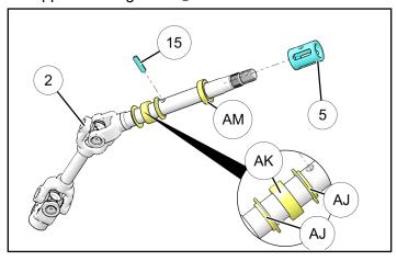
30. Slide lock collar ③ onto upper shaft ②, align hole and install spring pin ⑤.
