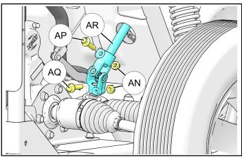
21. Remove fixed steering shaft (R) by pulling it through splash guard towards driver's seat as shown.
