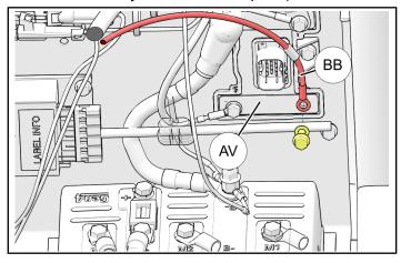
46. Connect Positive EPS Cable (9) to BMC (A) positive post as shown. Connect Negative EPS Cable (20) to BMC (A) negative post as shown.
