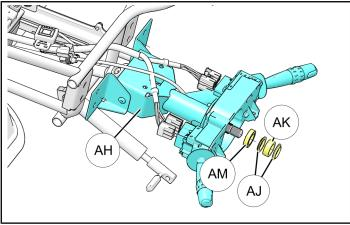
20. Remove lower steering shaft nuts  $^{(\!M\!)}$  and bolts  $^{(\!R\!)}$  and  $^{(\!M\!)}$ .
