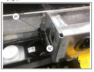
41. Plug in two connectors of EPS harness ③ to diagnostic port in front harness ⑥ and into blank plug ⑥.
