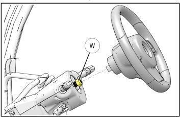
14. Remove steering wheel nut and steering wheel and set aside. Be careful to not break self-cancelling turn signal tab (3) on back of steering wheel.
