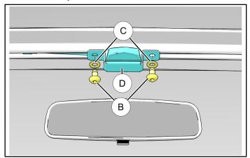
5. Remove light bracket assembly **D**. Disconnect connector for light housing **E**.
