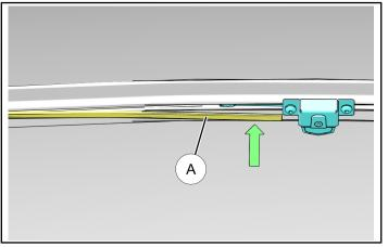
12. Install mirror ( by sliding base onto mount () from rear to front. Hand tighten screw ().
