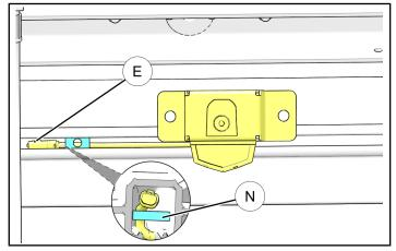
10. Ensure wiring is clear of mounting holes and mount bracket assembly <sup>(2)</sup> using retained screws
