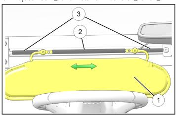
4. Once visor is properly located in t-slot, torque screws 4 to specification.
