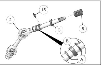
7. Slide lock collar (5) onto upper shaft (2), align hole and install spring pin (5).
