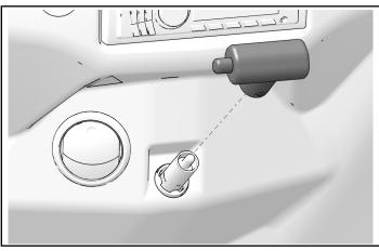
2. Install retained screw into parking brake handle. Hand tighten screw.
