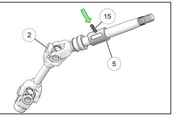
Insert steering column shaft <sup>(2)</sup> into retained steering column weldment and install assembly back to steel dash frame using four retained screws <sup>(b)</sup>. While installing, slide steering shaft <sup>(2)</sup> onto EPS unit <sup>(5)</sup> and ensure skip tooth is aligned with slit on U-joint. U-joint slits should align when installed. Torque four screws to specification.
