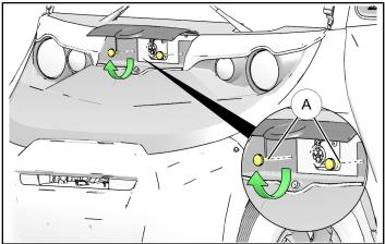
Slide hood down and away to remove from vehicle. Carefully set aside, ensuring hood is not damaged.
