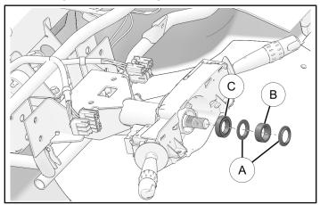
10. Loosely install bolt (1) and nut (1) into upper shaft joint but **DO NOT** tighten fasteners at this time.
