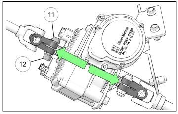
11. Reinstall retained upper steering column cover.
