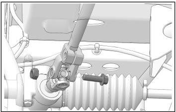
8. Remove fixed steering shaft by pulling it up and through splash guard towards driver's seat as shown.
