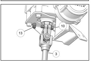
4. Install EPS with bracket and shaft into vehicle and secure with four bolts (8). Slip steering shaft onto rack during install. Torque to specification.
