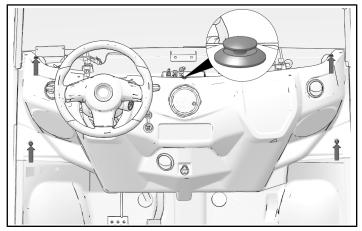
2. Disconnect any electrical connectors, switches, gauges, vents, or accessories that pass through lower dash panel and pull lower panel off vehicle.
