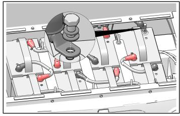
2. Ensure cable is set aside and will not make contact with negative terminal.
