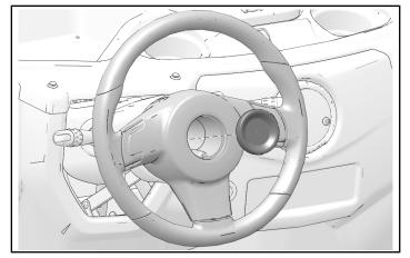
3. Loosen steering wheel nut leaving 2-3 threads engaged to steering shaft for next step. Make sure key is out of ignition as it will help to use steering lock to loosen steering nut.
