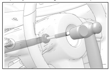
5. Remove steering wheel nut and steering wheel and set aside. Be careful to not break selfcancelling turn signal tab on back of steering wheel.
