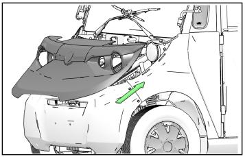
2. Open charge port door. Hand-tighten two knob screws (A) to secure hood to vehicle.
