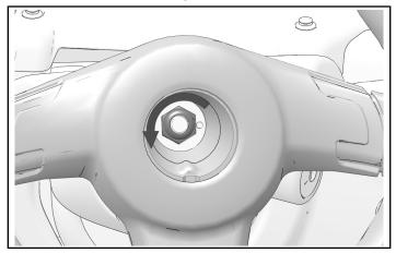
4. Center punch on steering shaft and make sure steering wheel nut (ii) is still on to prevent damage to steering shaft threads. Strike punch until you feel steering wheel pop off of steering shaft taper (usually this takes a large amount of force).
