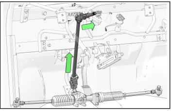
Remove nut and bolt from upper steering shaft joint. Slide upper shaft from joint. Slide steering shaft washers (A), bushing (B), and bearing (C) from upper steering shaft. Retain parts for reassembly.
