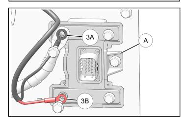
2. Route harness ③ following front harness. Secure EPS harness ③ to main front harness with cable ties ⑦.
