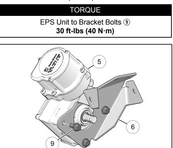
3. Install lower EPS steering shaft ① to EPS with screw ⑩ and nut ⑬ outside of vehicle. Make sure to align slit on knuckle with skip tooth on steering rack. Torque to specification.
