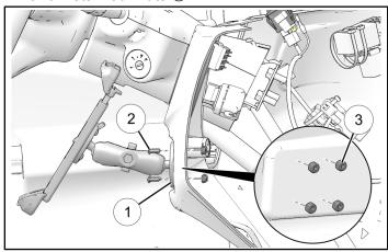
2. Counter hold nuts ③ and torque screws ② to specification.
