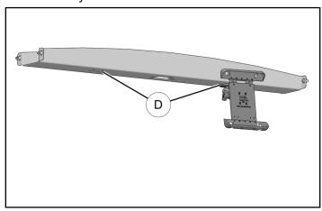
2. Hold tablet mount ① in place, insert four screws ② and install four nuts ③.
