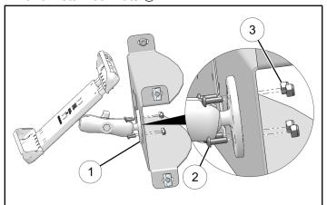
3. Counter hold nuts ③ and torque screws ② to specification.
