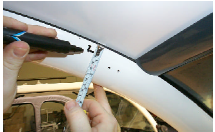
Fig. # 10 Mark roof rail 1/2" down from ceiling
