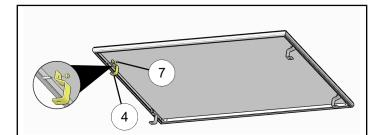
Keep distance 134 mm between bracket and inside of extrusion for all four brackets as shown.
