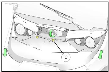
10. Mount solar charger ③ to chassis frame (D) using bolts <sup>①</sup> and nuts <sup>③</sup>. Torque nuts to following specification.
