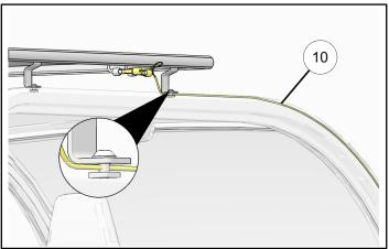
13. Cover solar panel harness with T–slot cover <sup>(1)</sup>.
