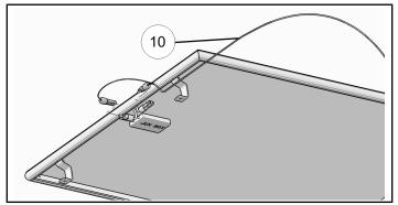
8. Use Panduit strap (1) to fasten solar panel harness (1) to front bracket (4) on RH side.
