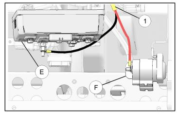
15. Connect solar harness 1 to solar charger 3 use panduit straps to hold in place.
