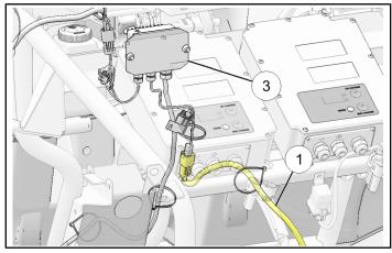
Route controller terminal ring (G) from solar charger along main vehicle harness (H) and fasten using Panduit strap <sup>(1)</sup>.
