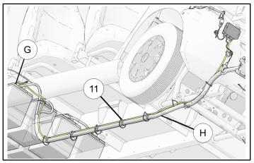
17. Reconnect battery connections disconnected in Step 2, connecting solar controller terminal ring (G) on top of the battery connection.
