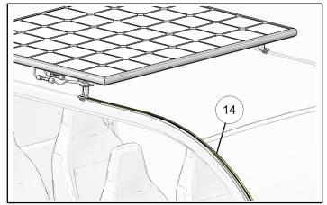
14. Connect solar harness ① to contactor assembly (PN 4012818) (F) with red wire and motor controller (PN 4015643) (E) with black wire.
