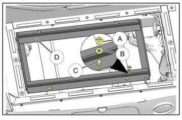
Install terminal mounting bracket ① to lithium ion battery tray ① with screws ⑥, washers ③, and nuts ②. Install terminal ⑦ to bracket ① with screws ③, washers ③, and nuts ②. Torque fastener to specification.
