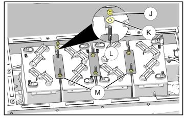
4. Remove old flooded batteries (1) or maintenance free batteries from battery tray.
