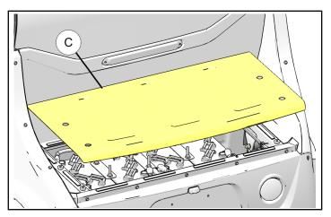
b. For eL XD: Remove six hex head screws (D) and three screws (E) to remove rear battery access cover (C).
