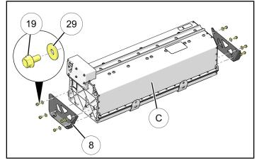
Install assembled batteries and brackets (a) onto battery tray (1) with screws (17), washers (28), and nuts (28). Note different positions for 12.4 kw battery pack and 8.9 kW battery pack.
