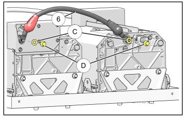
Install appropriate Li-Ion Harness by plugging large connector into Li-Ion Module. Now plug connector into large battery, remove blank plug from connector and plug into small battery. Connect small cable to positive battery terminal on small battery. Torque *ALL already connected* battery terminal connectors to specification.
