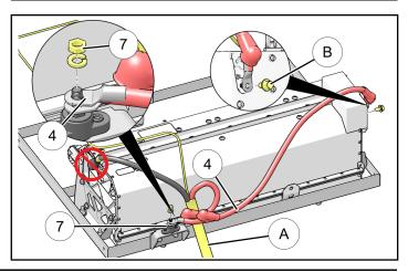
Install appropriate Li-Ion Harness by plugging large connector into Li-Ion Module and connector into large battery. Connect small cable to positive battery terminal on large battery. Torque *ALL already connected* battery terminal connectors to specification.
