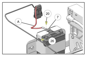
Insert battery nut <sup>(26)</sup> into negative battery post. Connect Negative 12V Battery Cable <sup>(5)</sup> to 12v battery negative post using supplied battery screw <sup>(20)</sup>. Route cable around rear along main harness as shown to main negative post. Torque screw to specification.
