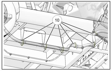
Plug lithium harness connector (A) into diagnostic port connector (B) and replace diagnostic port connector (B) with other lithium harness connector (C).
