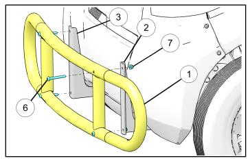
b. **Kit PN 2881629:** Install bumper ① to bumper brackets (LH ②, RH ③) using screws ⑥ and nuts ⑦ as shown. Torque nuts ⑦ to specification.
