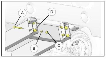
Install bumper brackets (LH 2), RH 3) to chassis tube using retained screws (A), washers (B), spacers (D), and nuts (C) as shown. Torque nuts (C) to specification.
